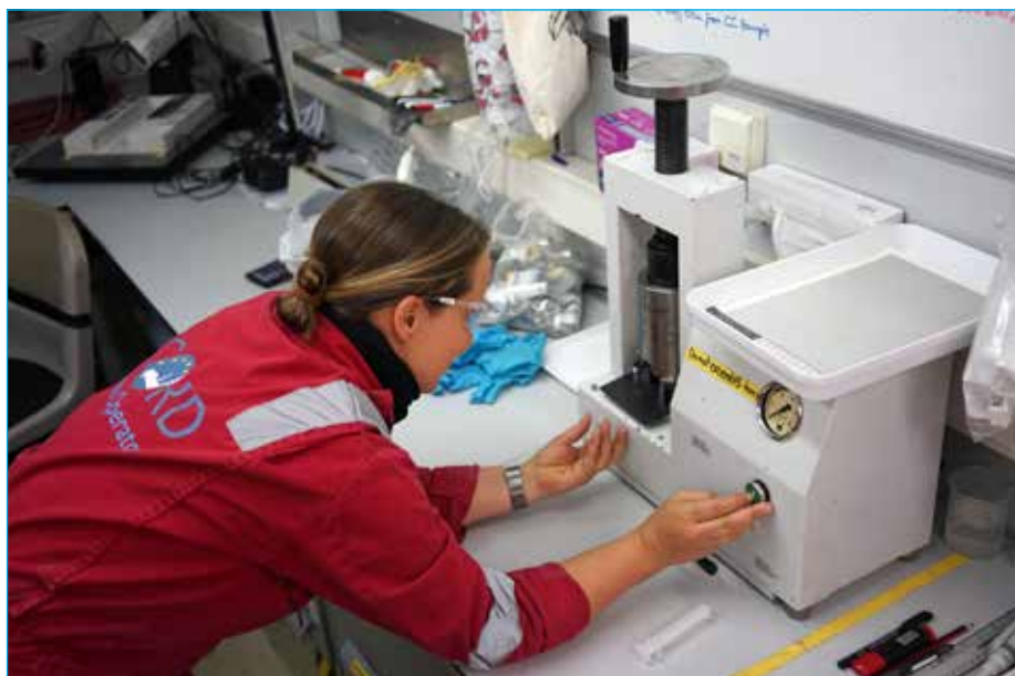
Luzie Schnieders collects pore-water samples from sedimentary cores during the offshore phase of Expedition 381 (photo E. Le Ber, ECORD/IODP).
