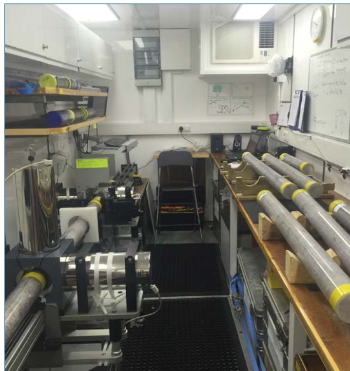
The multi-sensor core logger (MSCL) container busy with cores during the Expedition 364 (photo M. Rebolledo-Vieyra, ECORD/IODP).
