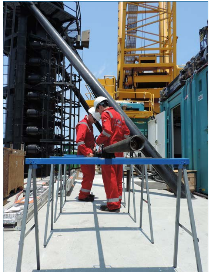
In preparation for downhole logging operations during Expedition 364, Gilles Henry and Laurent Brun, downhole logging engineers assemble a tool string of slimline probes (photo J. Lofi, ECORD/IODP).
