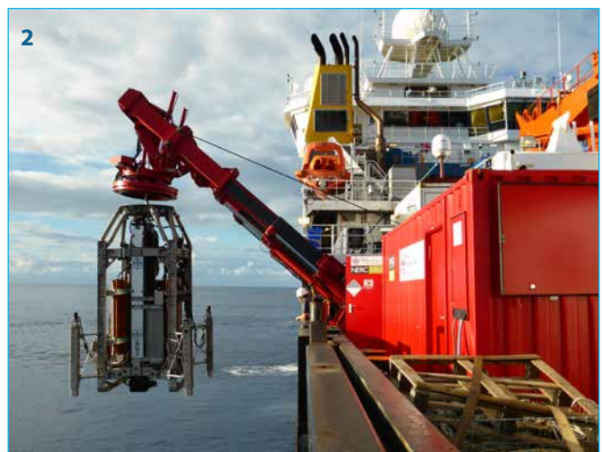
Seafloor drills onboard the RRS James Cook during Expedition 357: 1, deployment of the MeBo over the stern of the ship (photo Y. Morono, ECORD/IODP), and 2, recovery of the RD2 over the side of the ship (photo D. Smith, ECORD/IODP).
