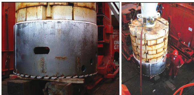
Figure 3. Views of the Drilling and Re-Entry Template (DART) which connects the ship to the seabed. The diameter of the dart cutting edge is 1.8m and the cutting edge is 30mm thick (Photos ESO/ECORD by D. Smith).
