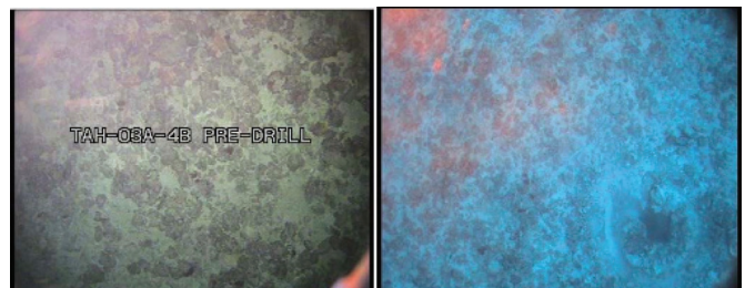
Figure 5 (left) shows the acceptable seabed pre-drill image. Figure 5 (right) shows the area after coring has taken place and shows the white ring of the template cutting edge and the dark area of borehole within it (Photos ESO/ECORD).
