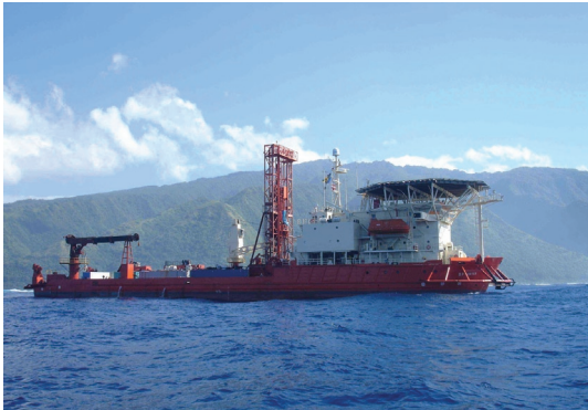
Figure 2. The DP Hunter, the dynamically positioned drilling platform used during the Tahiti Sea Level Expedition (Photo ESO/ECORD by I. Pheasant).
