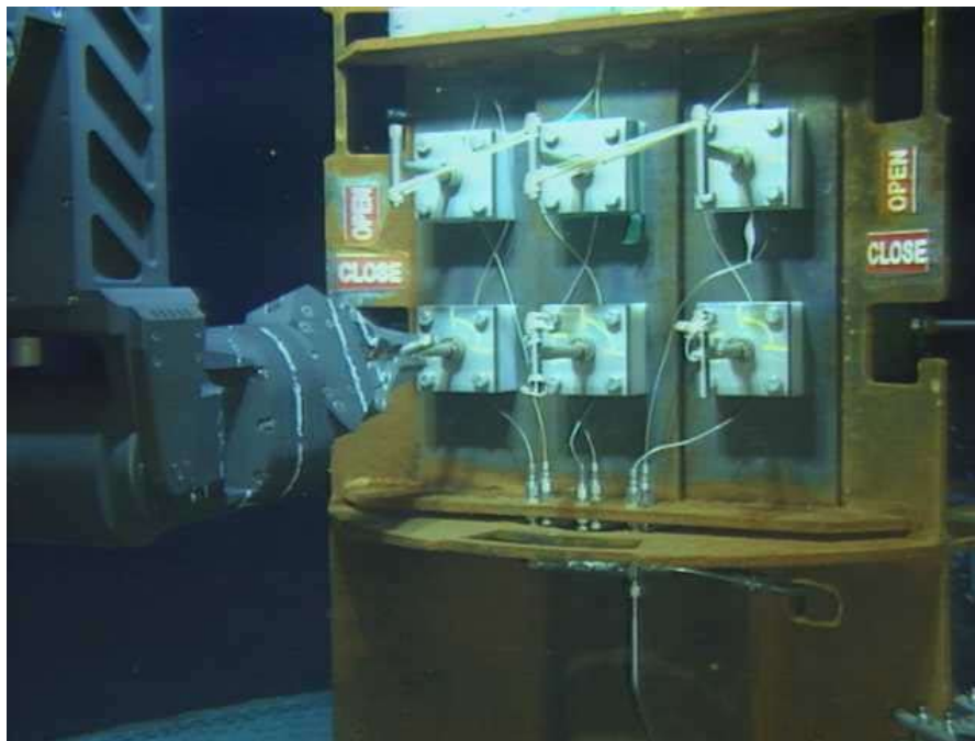
Figure 3. CORK observatory at the eastern flank of the Juan de Fuca Ridge. A remotely operated vehicle opens valves to retrieve fluid samples from a basaltic aquifer. (Photo by Geoff Wheat.)
