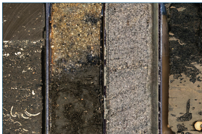
Photo 3: Various sediment lithologies - from silty clay to coarse-grained sand - recovered at different depths during the New Jersey Shallow Shelf MSP Expedition (© ECORD/IODP).
