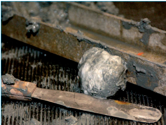
Photo 6 : A chunk of gas hydrate recovered from shallow depth (about 6 m below seafloor) at cold vent Site U1328 - Expedition 311(IODP/TAMU).
