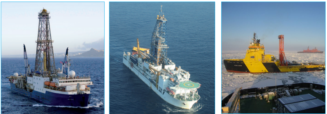
Photo 1: The three IODP drilling platforms. From left to right, the JOIDES Resolution (William Crawford, IODP/TAMU), Chikyu (©IODP/JAMSTEC) and the mission-specific platform the Vidar Viking used during the Arctic Coring Expedition in 2004 (D. McInroy ©ECORD/IODP).
