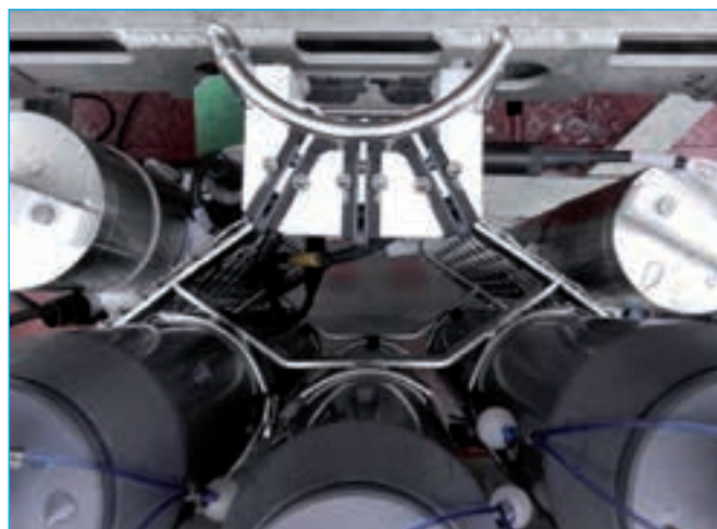
Seafloor drill-mounted sensor and water sampling assembly. Three water sampling bottles (grey) are visible. The two stainless steel cylinders house the various sensors mentioned in the main text. Water is pumped from close to the point of drilling to the sensors via flexible tubing (© ECORD/IODP).
