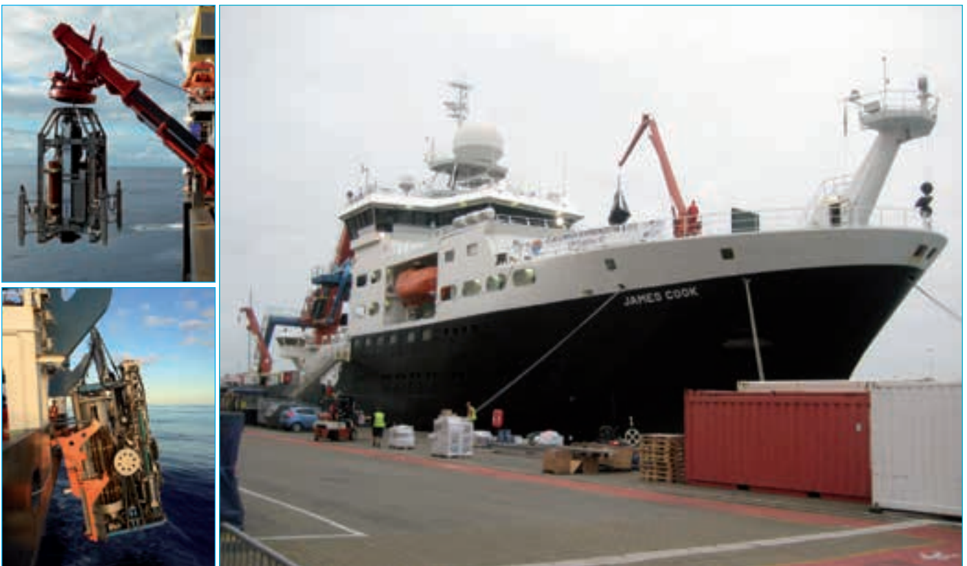
Top left, deployment of the BGS RD2 seafloor drill over the side of the RRS James Cook (D. Smith ©ECORD/IODP); bottom left, deployment of the MARUM MeBo70 seafloor drill over the stern of the RRS James Cook (D. Smith ©ECORD/IODP); right, RRS James Cook in port during mobilisation for Expedition 357 Atlantis Massif Serpentinization and Life (H. Kuhlmann ©ECORD/IODP).
