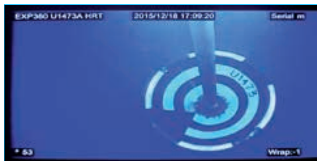
Expedition 360: The reentry cone being tripped down before release (Christopher MacLeod & IODP).
