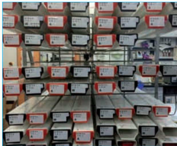
Cores of Expedition 357 Atlantis Massif Serpentinization and Life during the Onshore Science Party. Working halves are identified by black caps, archive halves by red caps (© ECORD/IODP).
