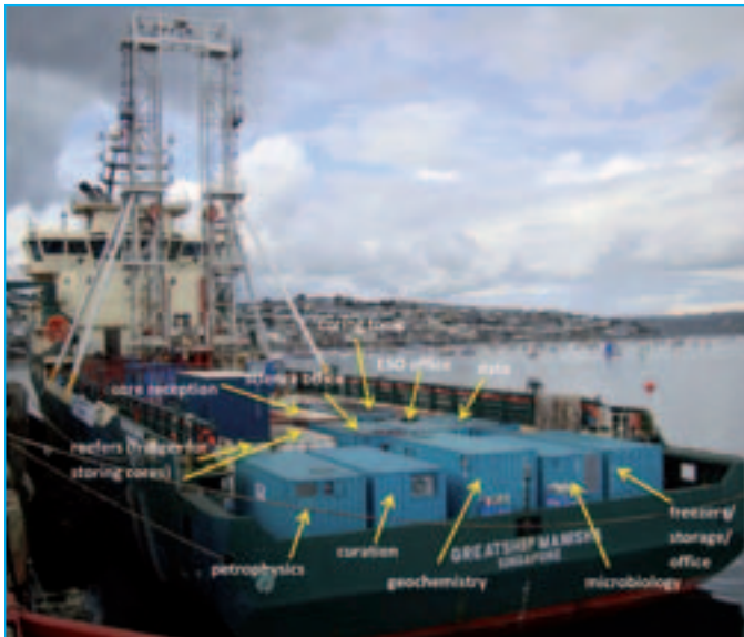
The Greatship Manisha equipped with the drill rig and ESO containers during mobilisation in Falmouth, UK (D. Smith ©ECORD/IODP)
