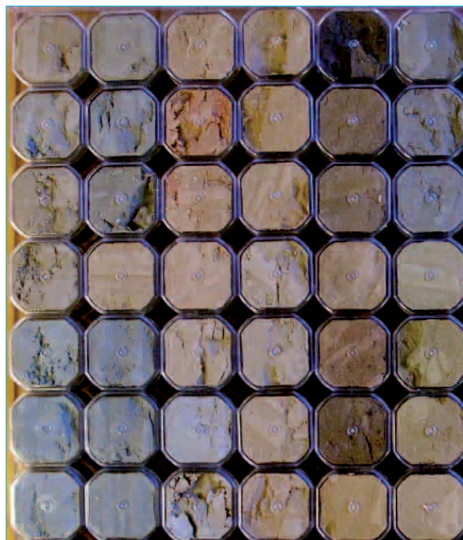
Core samples for paleomagnetic measurements (cryogenic magnetometer) during Expedition 342 (photo Peter Lippert IODP/TAMU).
