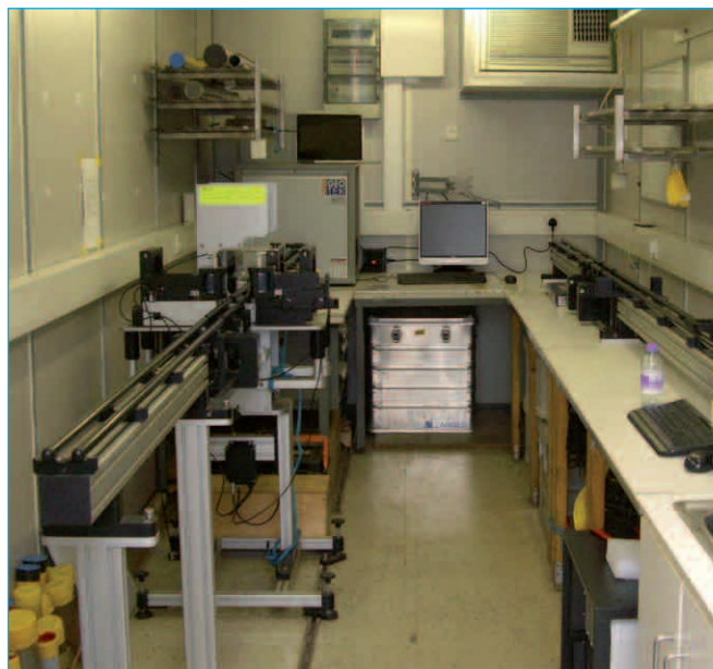
The refitted Petrophysics Container ready for IODP Expedition 347. The new MSCL 152 is desk-mounted on the right (photo taken by John Roberts, Geotek).
