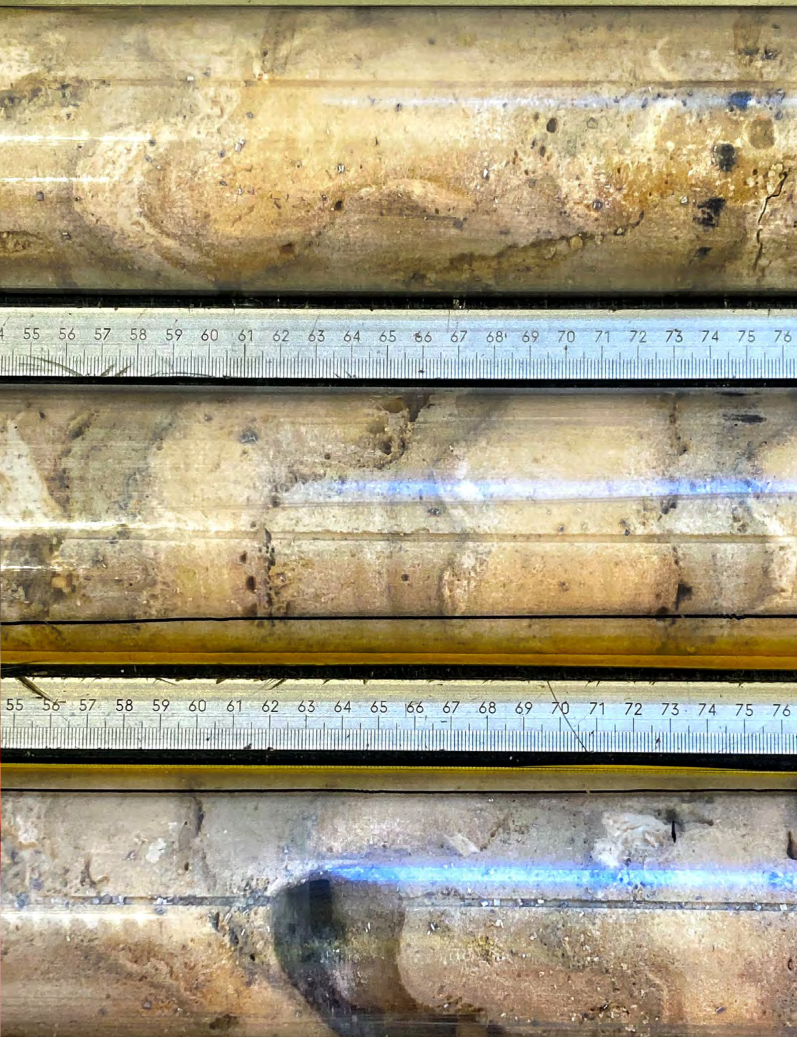
Freshly recovered core sections onboard MMA Valour during Expedition 389: fossilized reef deposits after they have been placed in plastic core liners. The different colors and textures represent various corals, algae, and microbialites from the fossil reef. . Credit: M. Parker, ECORD/IODP.
