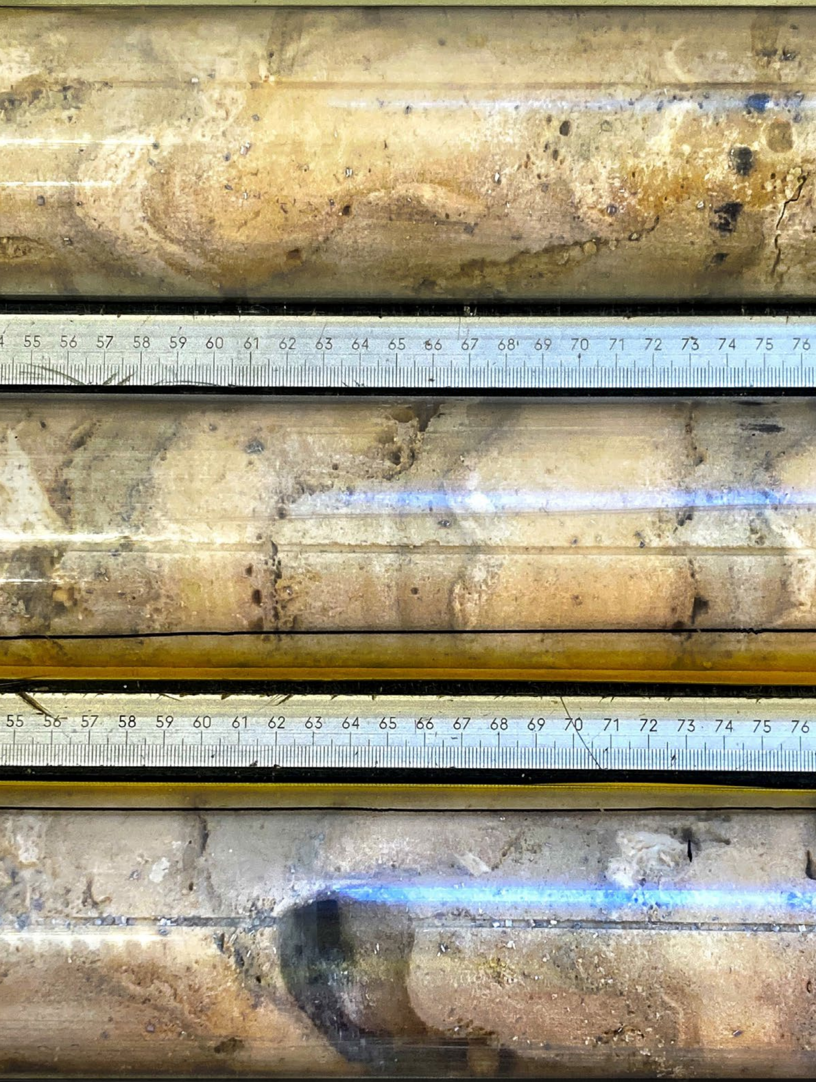
Freshly recovered core sections onboard MMA Valour during Expedition 389: fossilized reef deposits after they have been placed in plastic core liners. The different colors and textures represent various corals, algae, and microbialites from the fossil reef. Credit: M. Parker, ECORD/IODP.
