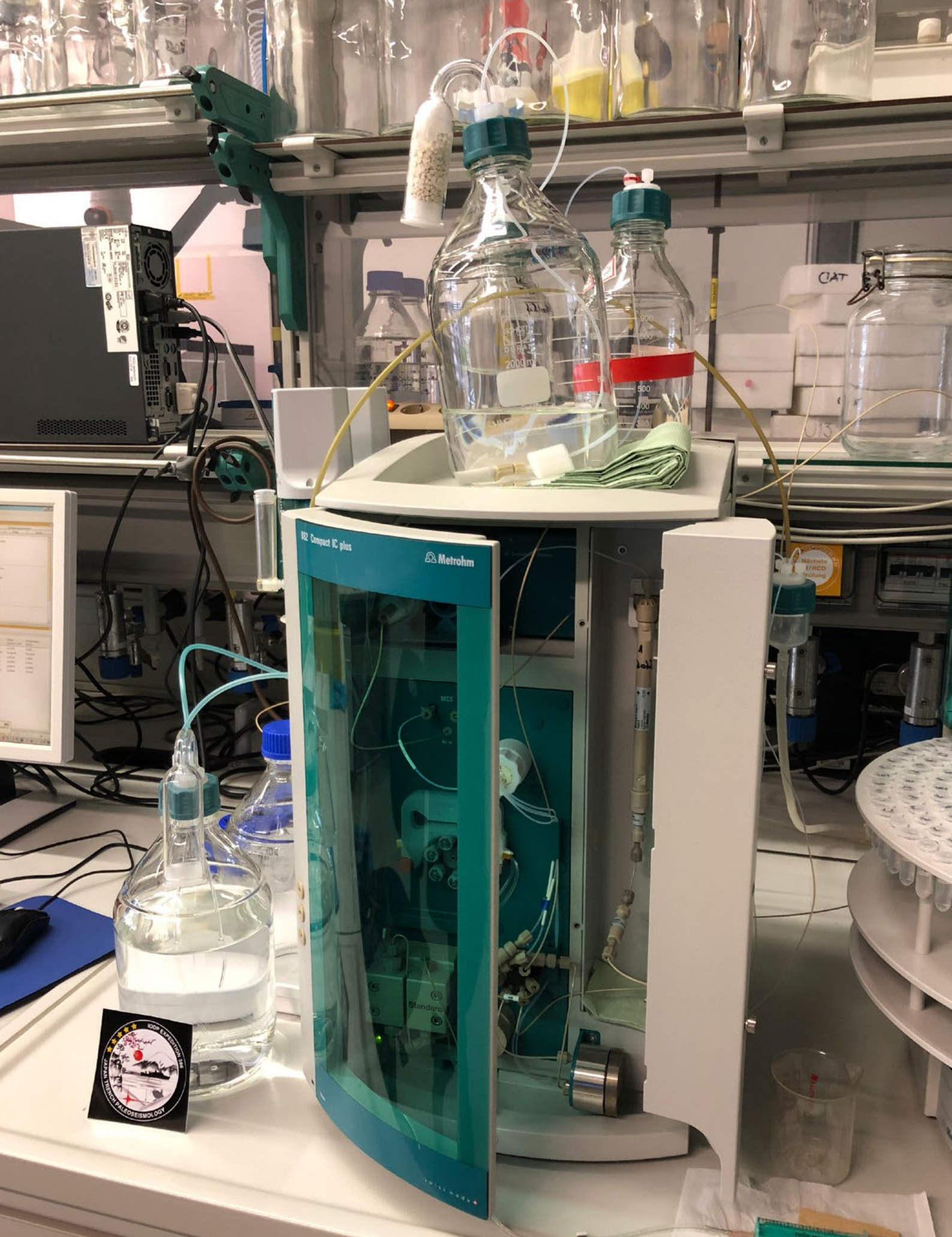
Ion Chromatograph was used to measure the sets of samples that arrived at Bremen Core Repository from IODP Expedition 386 OSP that took place onboard D/V Chikyū , Japan. Credit: U. Prange, ECORD/IODP.
