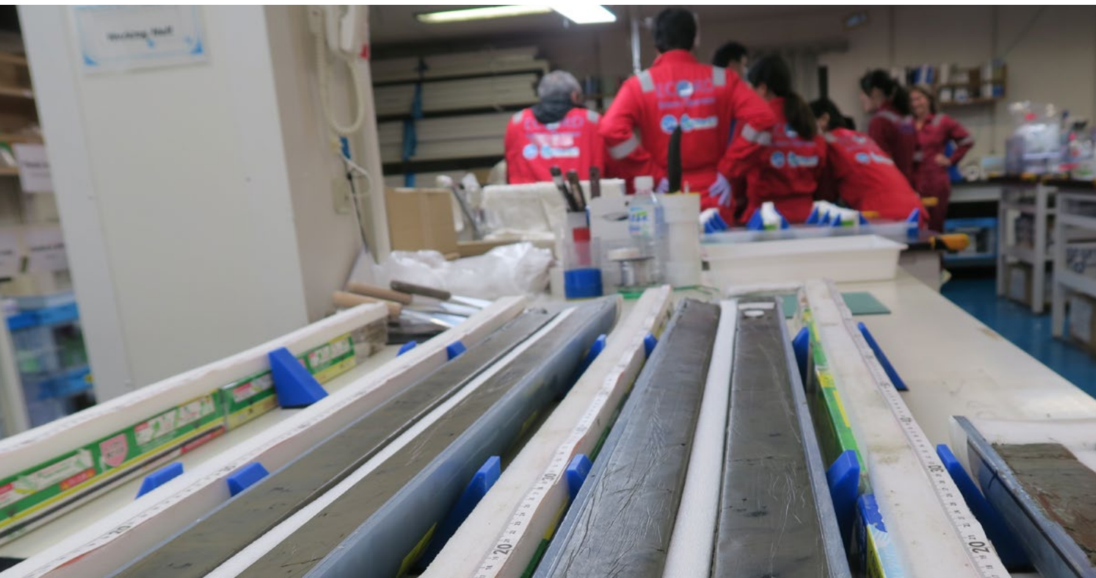
Splitting cores during PSP for IODP Expedition 386 onboard Chikyu . Credits: M. Mowat, ECORD/IODP/JAMSTEC.
