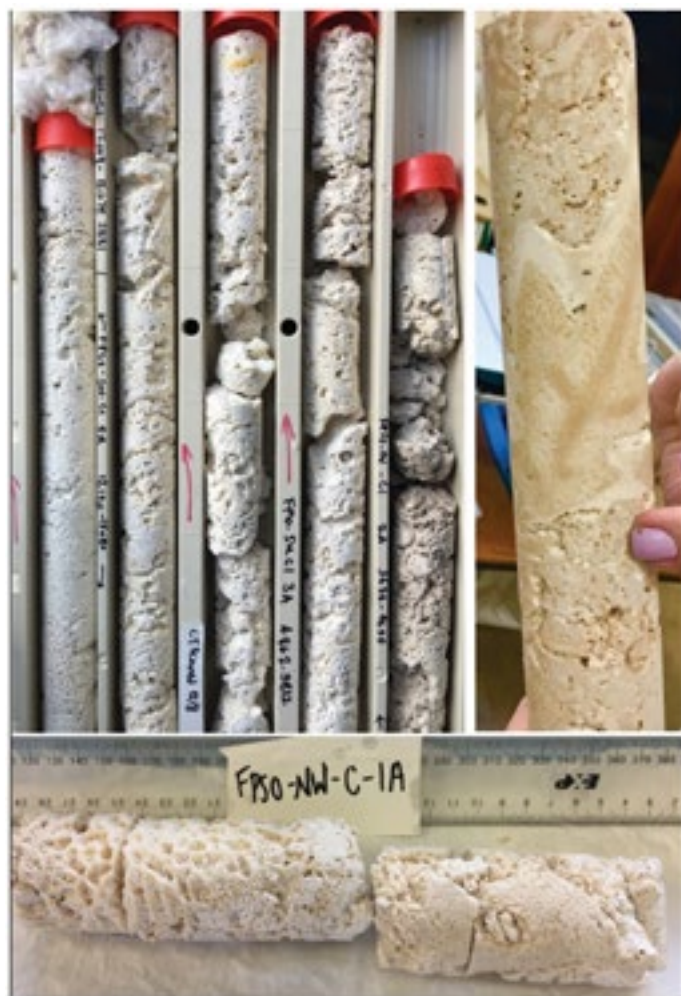
Fig. 4. Representative core images showing the high quality core recovery in a range of very challenging fossil reef lithologies using a sea bed rock drill (Webster et al., In Press 10/09/21). These MIS 3 to 4 reef cores were recovered from the North West Shelf of Australia using the seabed drilling system PROD in ~80 m water.
