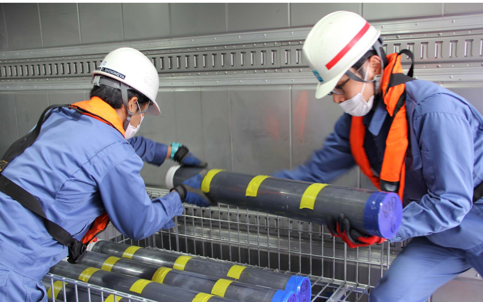
Arranging the cores onboard R/V Kaimei during IODP Expedition 386. Credits: N. Okutsu, ECORD/IODP/JAMSTEC.
