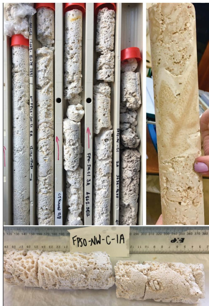
Fig. 4. Representative core images showing the high quality core recovery in a range of very challenging fossil reef lithologies using a sea bed rock drill (Webster et al., In Press 10/09/21). These MIS 3 to 4 reef cores were recovered from the North West Shelf of Australian using the seabed drilling system PROD in ~80 m water.
