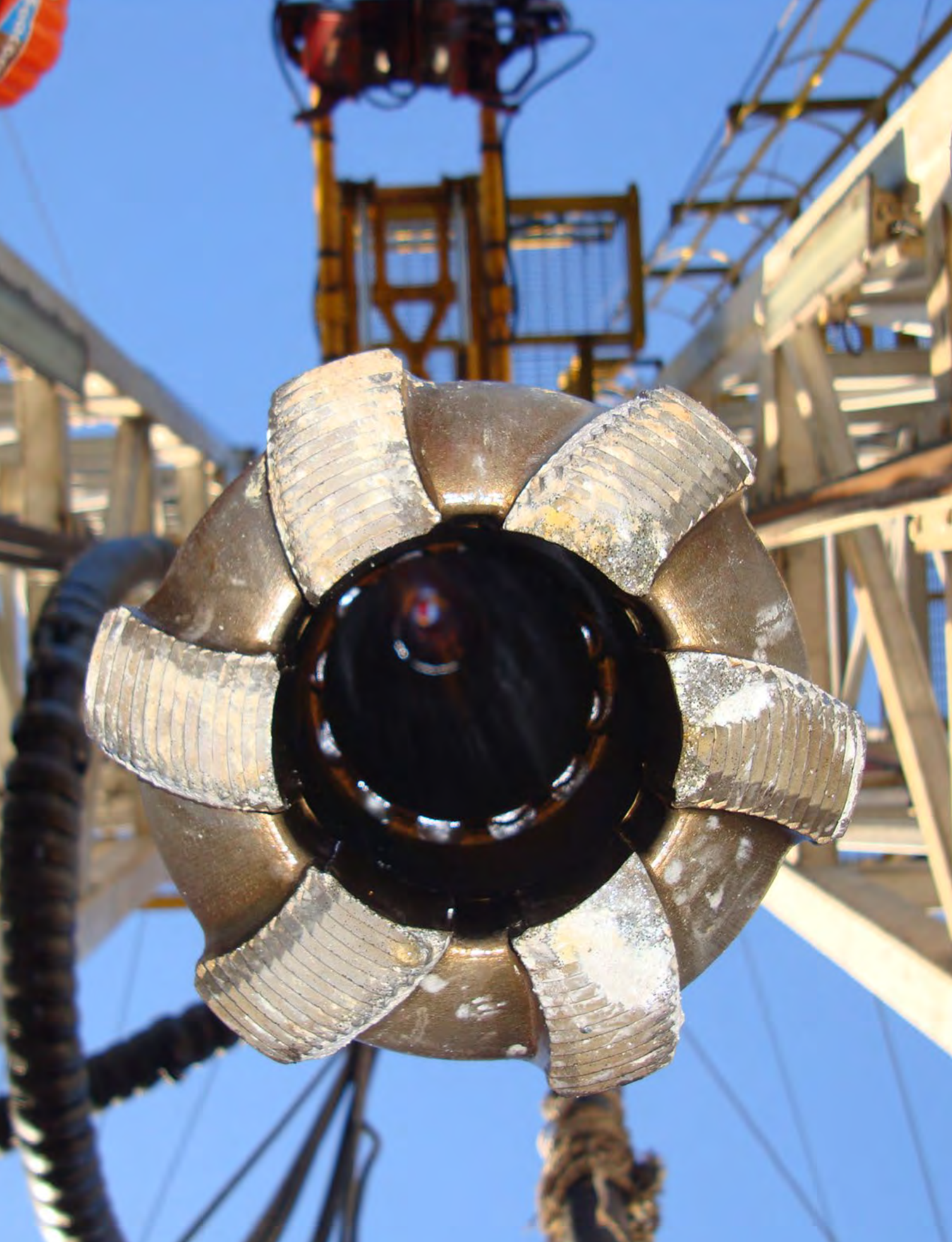
Drill bit, IODP Expedition 325 (photo D. Smith, ECORD/IODP).
