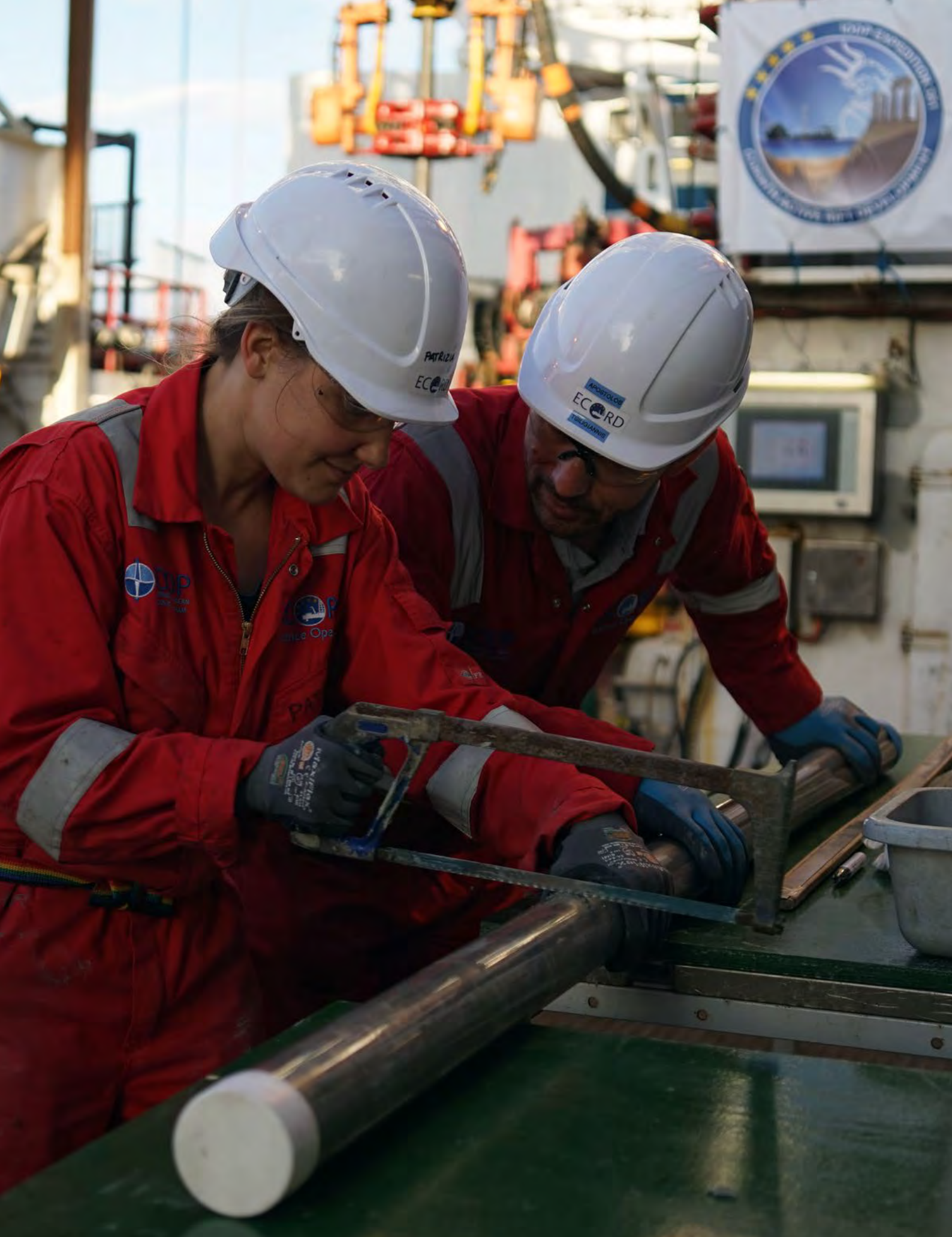
Patrizia Geprägs (ESO) cutting a freshly retrieved core during IODP Expedition 381 (photo E. Le Ber, ECORD/IODP).
