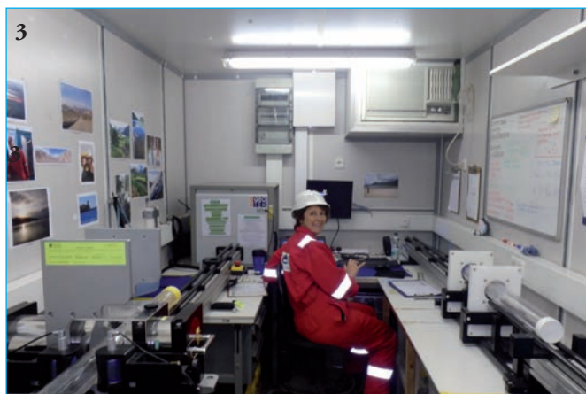
3 Dual MSCL set up in the ESO Petrophysics container with Anette McGrath (©ECORD/IODP).
