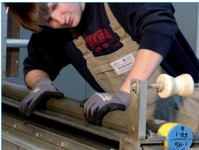
Splitting of an Expedition 347 core (Nils Monsees, student assistant, Bremen University (C. Cotterill ©ECORD/IODP).
