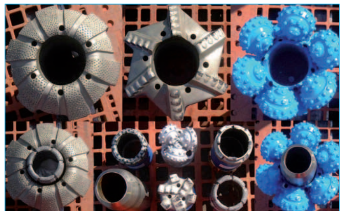
Examples of drill and core bits from the BGS Marine Wireline Coring System, to allow for effective coring in any formation encountered.
