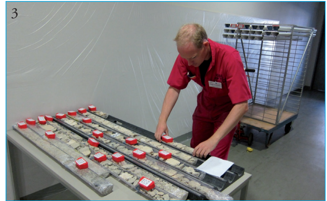
Figure 3: Holger Kuhlmann, ESO assistant lab manager at MARUM, displays the archive halves after the cores were split.
