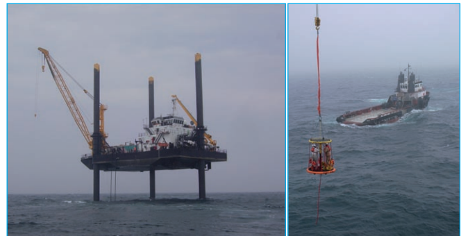
Figure 4: The Kayd on site ready to start drilling; Figure 5: The basket transfers scientists to the Kayd . (© ECORD/IODP).
