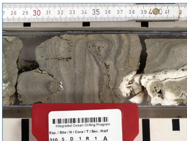
Figure 1. Laminated and thrombolitic carbonate crusts in the Tahiti reef, referred to as microbialites (photo ECORD/IODP).
