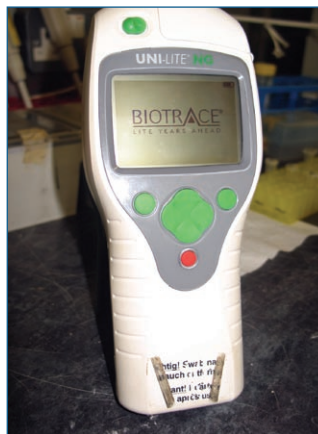
Figure 2. The new, handheld ATP analyzing instrument, manufactured by UNILITE, which was used to detect the presence of life with a swab-test during shipboard analysis of core surfaces (photo R. Warthmann).
