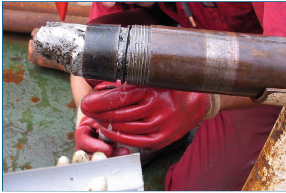
Figure 4. Possible sources of microbial contamination: contact with the operator's gloves, drill water and/or drill pipe (photo ECORD/IODP).
