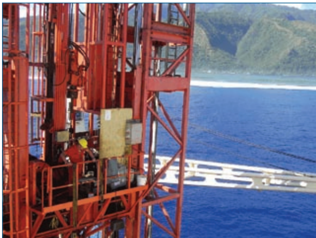
Figure 1. Petrophysics staff scientist in the rooster box. The acquisition of downhole geophysical data was done in the rooster box which, in the used piggy-back drilling system, is heave-compensated. Although logging conditions were quite adverse (hot and humid), it did provide a work environment with a brilliant view (IODP photo).
