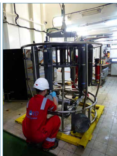
Expedition 357: First CTD cast at site M0068 with water sampling on recovery (photos C. Cotterill © ECORD/IODP).
