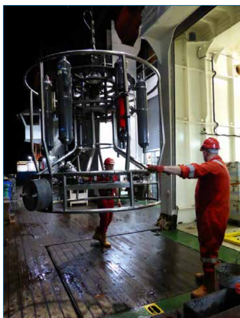
Expedition 357: First CTD cast at site M0068 with water sampling on recovery (photos C. Cotterill © ECORD/IODP).
