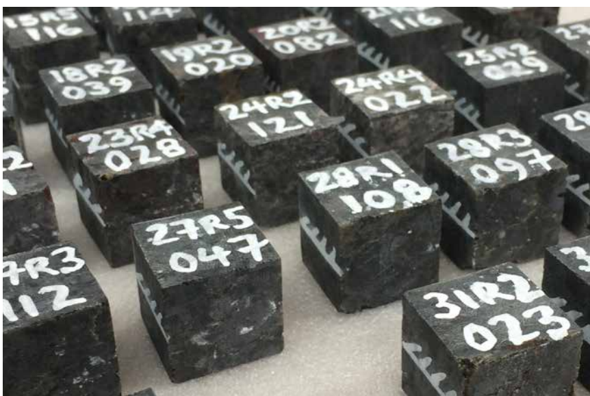
Figure 2: Cubic discrete samples awaiting paleomagnetic analysis, IODP Expedition 360 SW Indian Ridge Lower Crust and Moho (Antony Morris & IODP).
