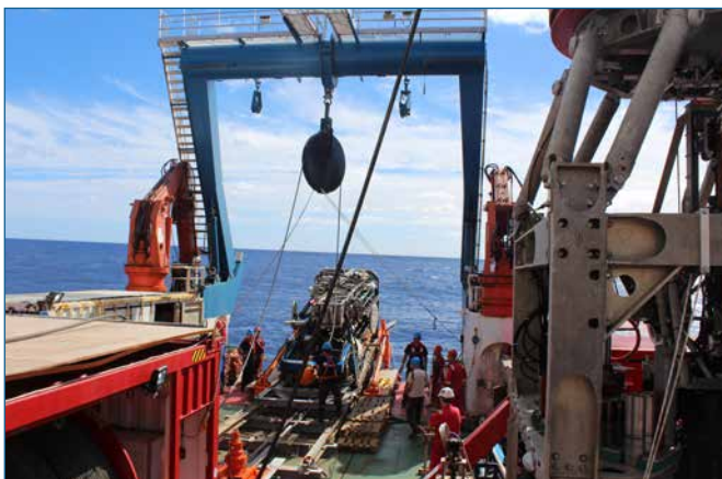
Left, deployment of the MeBo over the stern of the RRS James Cook (photo Y. Morono © ECORD/IODP); right, recovery of the RD2 over the side of the RRS James Cook (photo D. Smith © ECORD/IODP).
