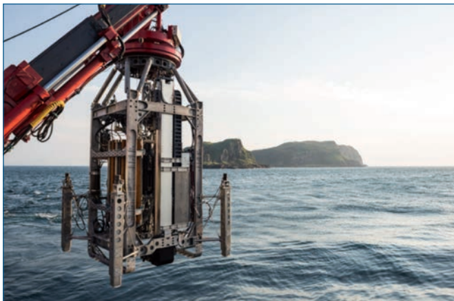
Launch of the RD2 seafloor drill, offshore Oban, Scotland, during the recent trials.
